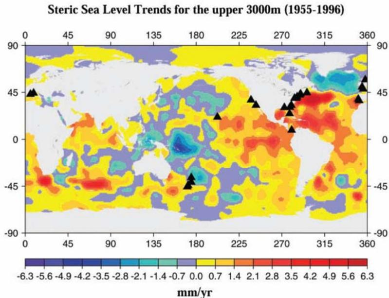
**Fig. 4.** Map of the geographical distribution of thermosteric sea level trends for 1955–96 computed with temperature data from (3) down to 3000-m depths. Black triangles show the locations of the 25 tide gauges.
