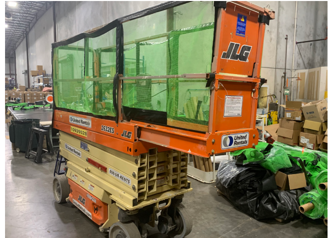
A MEWP (Mobile Elevating Work Platform) rigged with a DOPS (Dropped Object Prevention System). Courtesy of Forrest Hester, CEO of Tutus.
